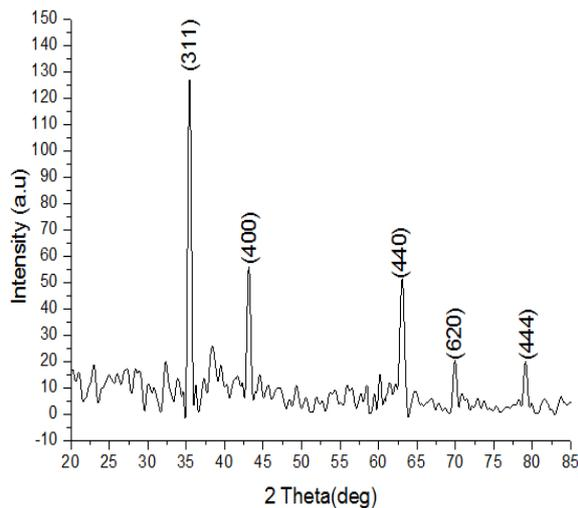
**Figure 1.** The XRD diffraction pattern of the MgFe<sub>2</sub>O<sub>4</sub> nanoparticle
